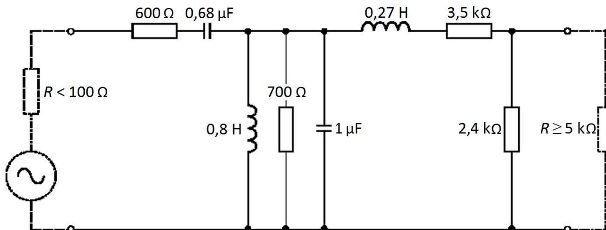
Figure B.3: White Filter circuit
